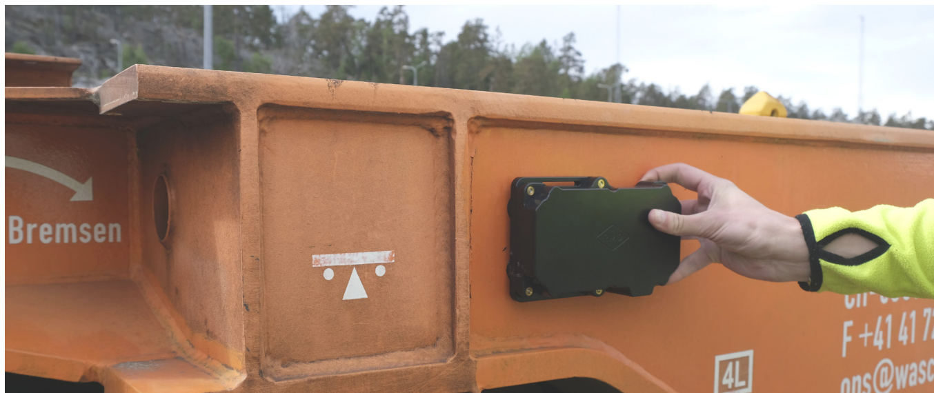
Performance Monitoring Unit (PMU)
