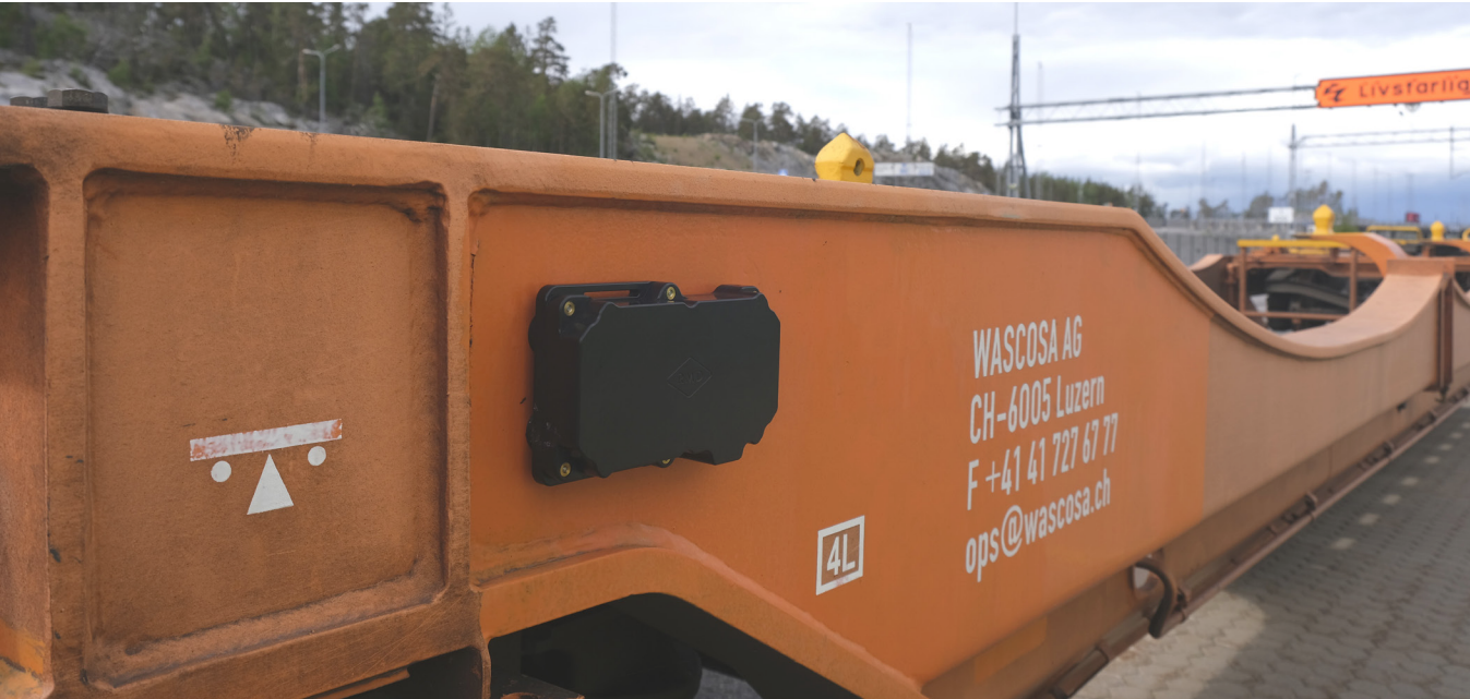
Performance Monitoring Unit (PMU)
