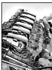
Scania's high-torque 450 or 490 horsepower 13-litre engines are now available in versions that can be operated on 100 percent biodiesel.
