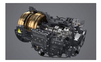
Scania's electric machine GE281 is a truly innovative solution for hybridisation of heavy trucks. By coupling two electric motors in a common housing with the core parts of Scania's latest Opticruise gearbox generation (via a dual input shaft), a unique solution was created. With continuous power of 230 kW and a gearbox PTO, it has the capacity to power various truck applications without having to engage the combustion engine.
