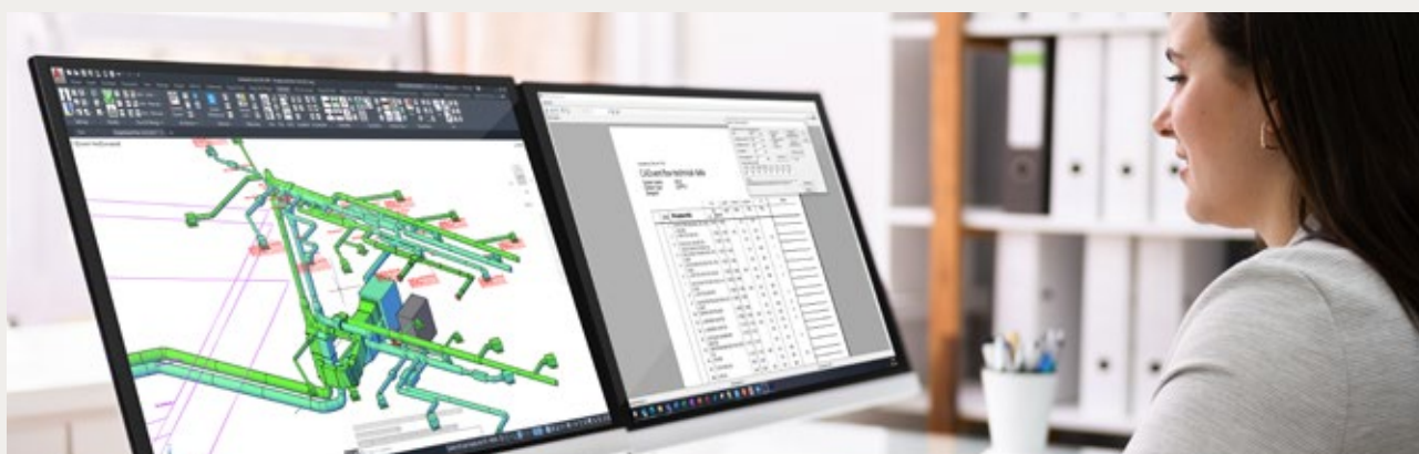
With the Lindab Quick Selection Tool (LindQST), customers can easily calculate sound levels, pressure drops and flow conditions.
