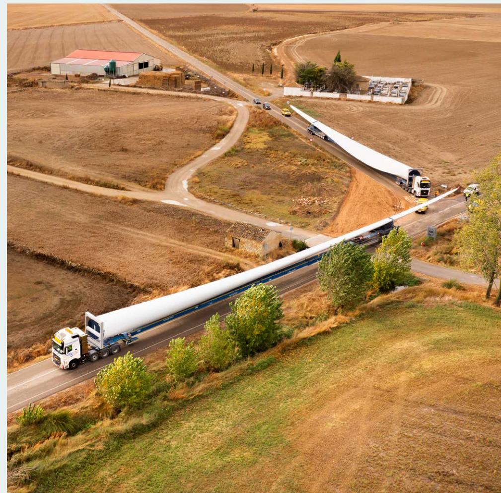
↑ Vestas V163-4.5 MW wind turbine blades being transported from the Daimiel factory in Spain..
