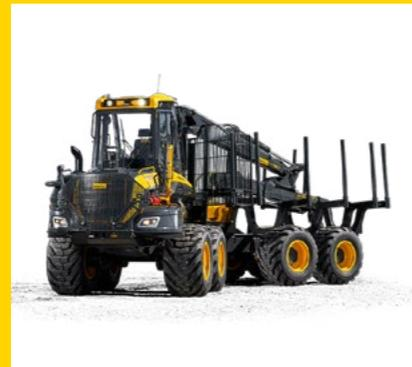
All PONSSE forwarder models have more than enough power for changing conditions and difficult terrain types. In addition to the regular hydrostatic transmission, PONSSE forwarders are equipped with CVT transmission that enables lower fuel consumption and higher tractive force.
