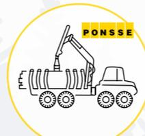
2. A PONSSE forwarder transports each assortment to its pile on the roadside.
