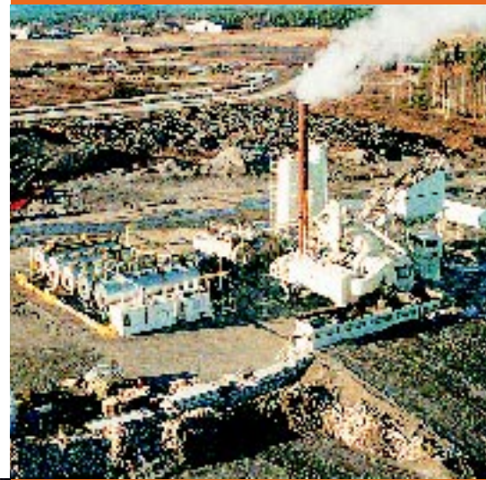
Above: The Veidekke Group is carrying out the paving of the eastern and western runways at the new main airport at Gardermoen. The photograph shows some of the Group's production equipment: the PMB plant (polymer modified bitumen) and an asphalt plant.
