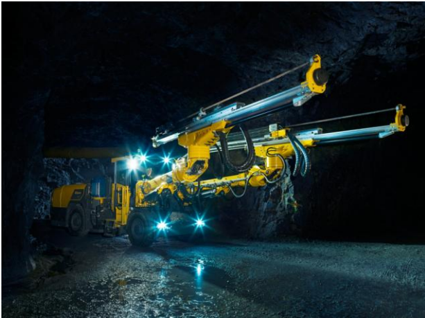
The Boomer M20 S face drilling rig is part of the order by MMG.
