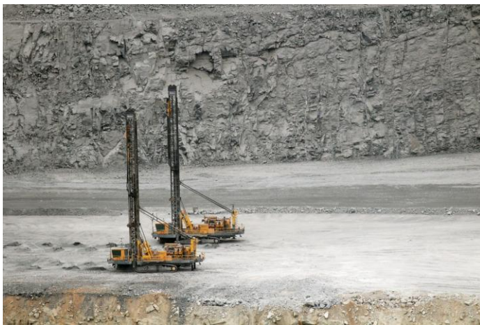
The Epiroc Pit Viper 351 blasthole drill rig
