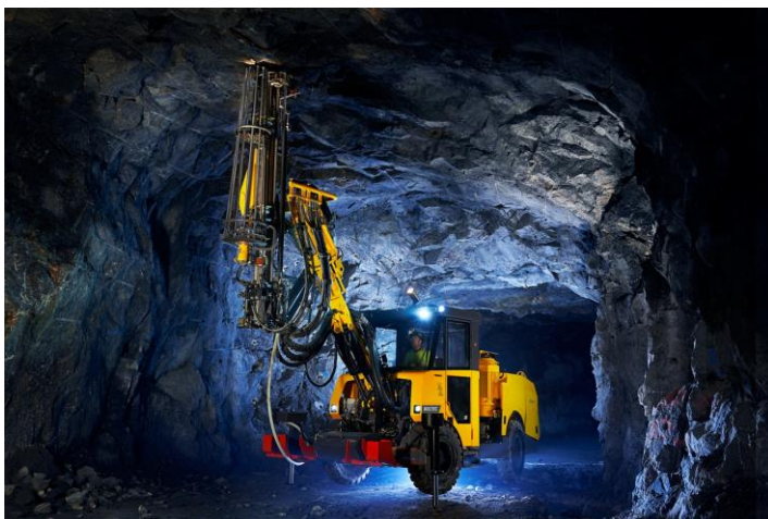
Epiroc’s Boltec S rock-reinforcement rig is part of the order by Dumas
