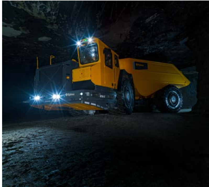
One of our most popular machines underground is the Minetruck MT42. It is a high speed 42-metric tonne truck, featuring state-of-the-art levels of safety and operator comfort which results in unmatched performance in underground mining and construction operations. Epiroc also offers a battery-electric version.
