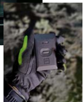
Epiroc offers various Mobilaris tags that enable the effective localization of personnel and mobile assets (such as vehicles or machinery) within a Wi-Fi or LTE network.
