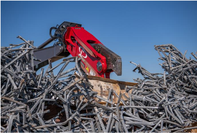
A Stanley Infrastructure mobile shear attachment for scrap recycling of the LaBounty brand
