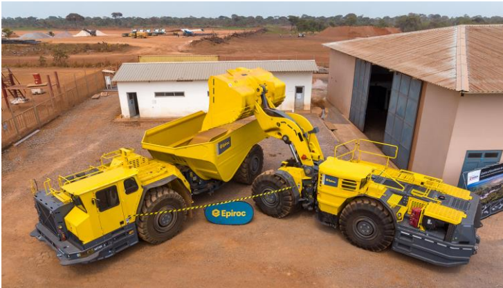
Epiroc's Minetruck MT65 S hauler and Scooptram ST18 S loader at Kamo-a-Kakula.
