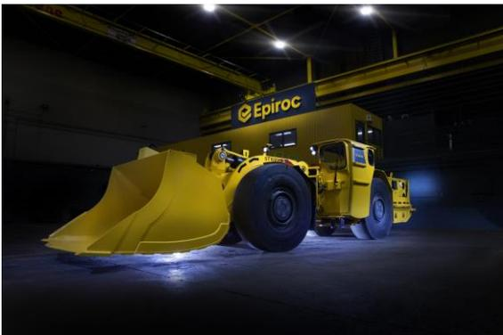
*A previously diesel-powered Epiroc Scooptram ST1030 loader converted by FVT Research into battery electric*
