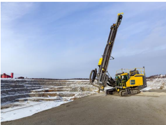
An Epiroc SmartROC D65 surface drill rig for quarrying and mining, one of the machines made by the Surface and Exploration Drilling division in Örebro, Sweden.
