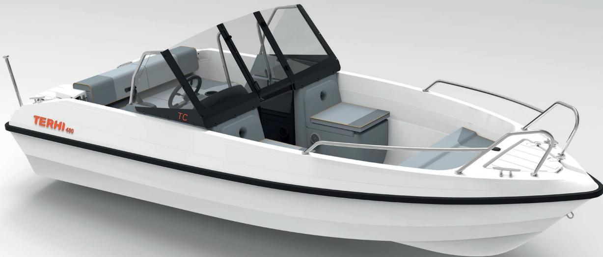
Boat's hull is made from ABS plastic with a three-layer structure. The unique construction of Terhi boats guarantee besides unsinkability, also quiet rides even in rough weather. The space in between the thermo-formed ABS-plastic hull and deck section is filled with non-water-absorbent polyurethane foam. The result is a solid and stiff sandwich construction, which is easy to maintain and quiet in use.
