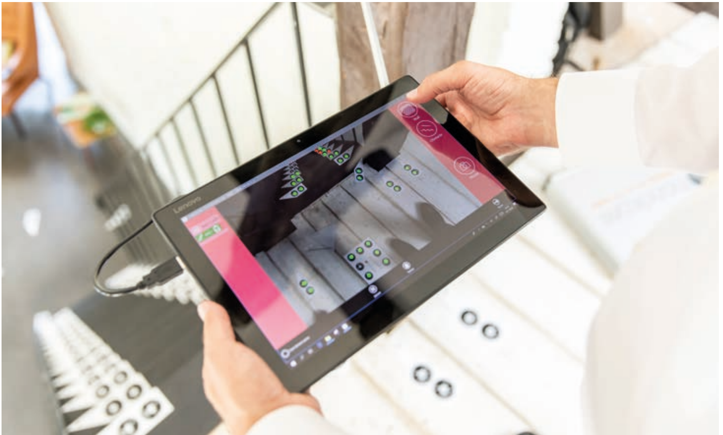
Photosurvey4D, a quick and easy staircase measurement tool.
