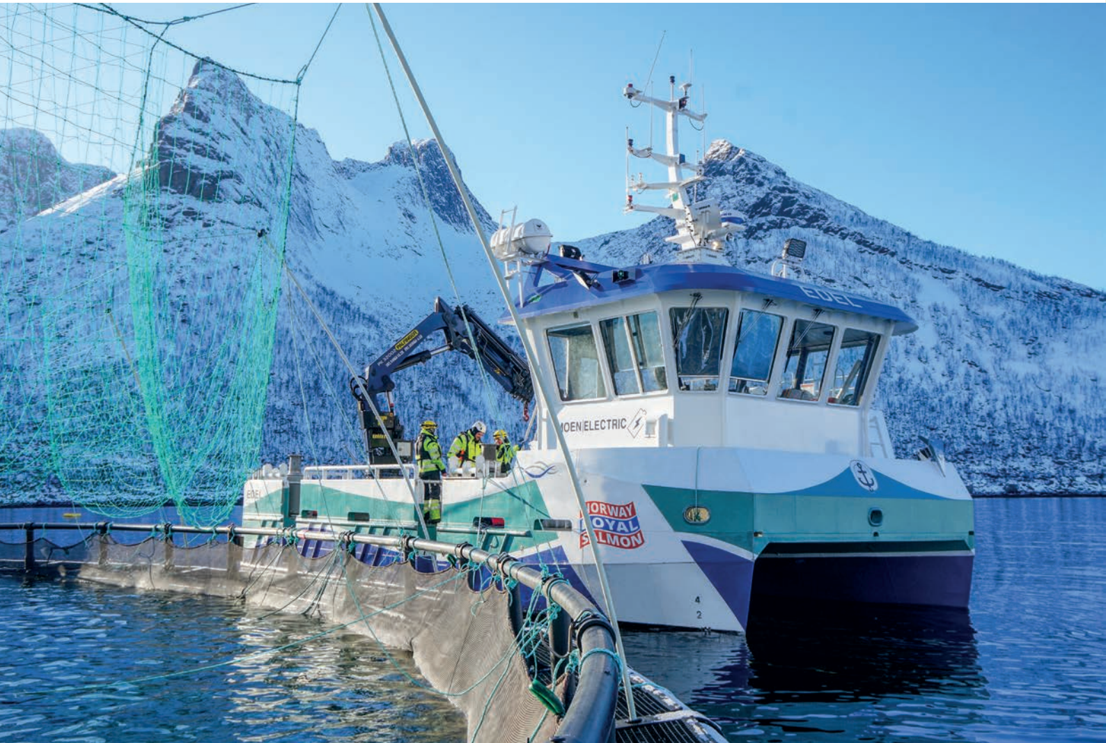
NRS's first hybrid boat, "Edel", is a diesel-electric catamaran that can reduce diesel consumption by 60 per cent.
