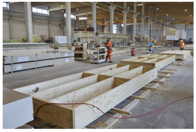
Lapwall also believes in the logic and assembly chain approach that have been adopted from the automobile industry: in industrial wood construction, the work steps are clustered together and prepared in advance. All that remains to be done on the building site is to connect the parts.
