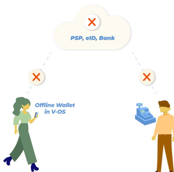
Figure: Crunchfish's trusted Offline Wallet application is implemented in a secure element in the consumer's mobile payment application.
