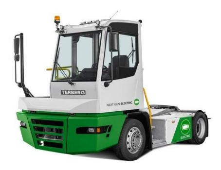
Terberg's electrified terminal tractor YT203-EV. The temperature controlled batteries (TMS) can be used in both hot and cold environments. With a fast charger that can deliver up to 150 kWh per hour, batteries of the strongest battery type are charged in just one hour.
