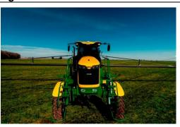
Caiman's recent first export to Australia – an Allison-equipped, self-propelled sprayer featuring a 3,650-litre tank, a working width of 36 metres and a 1.5-metre clearance.
