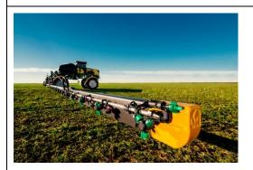
The self-propelled sprayer mists planted fields with fertilisers and other liquids and features an Allison 2500 fully automatic transmission.
