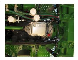
Caiman has been equipping machines with Allison Automatics featuring Continuous Power Technology™ for over a year, delivering superior performance with uninterrupted power to the drive wheels.
