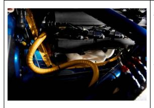
Ability to apply real gold onto ceramic creates innovative coating with 98% reflectivity, yet still insulates against heat in both heatshield and plasma sprayed coating variants.
