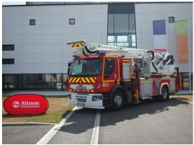
Built on a Renault Premium 340.19D chassis, with five-seat cabin, the aerial platform vehicle is equipped with a 247 kW engine and an Allison 3200 fully automatic transmission.
