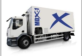
The MDX-1 comes equipped with two shredding units powered by the Allison transmission's dual PTO provisions.
