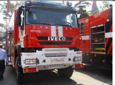
The PSA Chelnok fire engine is a rescue shuttle intended to provide first response, aid, and the gathering and evacuation of victims in emergency situations in tunnels.
