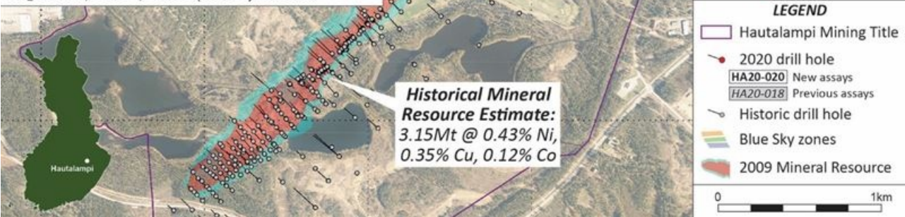
Figure 1. Drill hole collar plan for Hautalampi Project. Drill holes recently completed highlighted by red dots. Location of cross-section in Figure 2 highlighted by yellow triangles (section 47).
