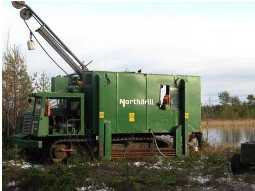
Figure 3. Northdrill Oy drill rig manufactured to operate year round in Finland.
