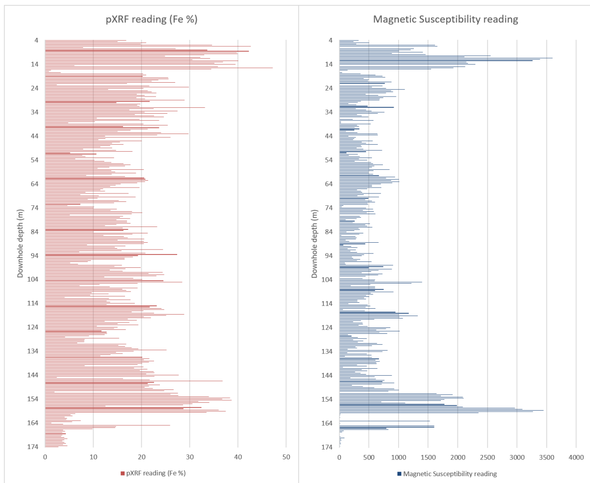
Figure 3: Portable XRF and Magnetic Susceptibility analysis. Note: these are spot measurements so only provide an indication of mineralisation.
