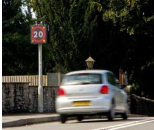
Messagemaker have developed a new electronic speed reduction safety sign, which has already been installed on numerous roads outside schools. These signs use the latest LED technology and enable remotely programmable timers to be set to 20 mph speeds during school hours, returning to normal speed limit signs at other times. The signs can also be configured to revert to Vehicle Activated Speed Signs outside of the core School Times.
