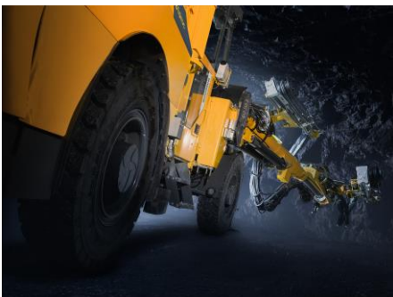
The battery-powered Epiroc Boomer M2 Battery drill rig
