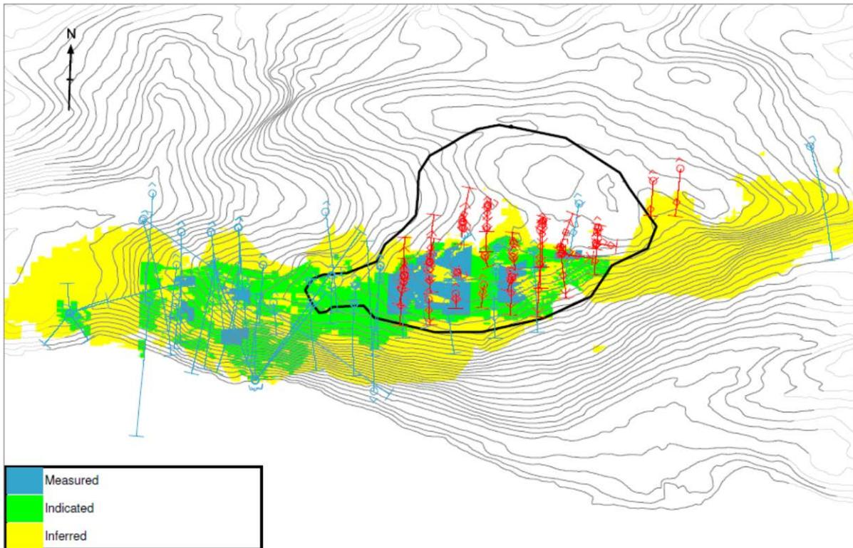
Figure above is the 2016 model, while the figure below is the 2008. The blue lines mark the historical drillholes and the red lines show the holes from the 2016 campaign. The solid black line marks the regulated open pit area.
