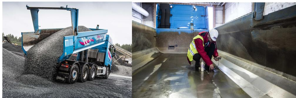
*The dump body in the pictures is made with Hardox® 500 Tuf in the bottom plate. It has transported over 40,000 metric tons of crushed rock during more than a year with very low wear. Measuring the thickness at the end section of the 6 mm bottom plate showed an average wear of only 5%.*
