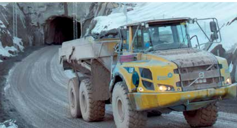
Trucks carry the ore up to surface via the ramp.
