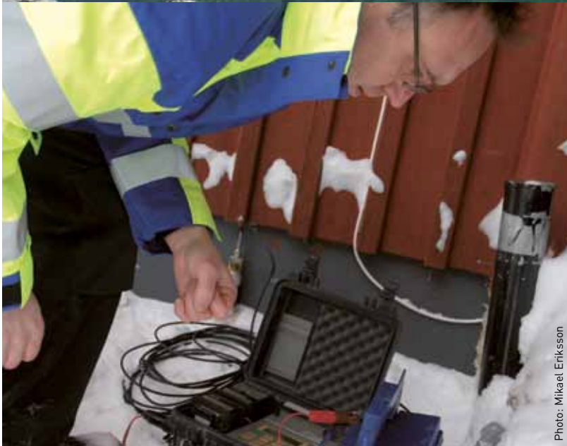
Vibration meters have been installed at some properties in order to check the size of tremors caused by underground blasts.
