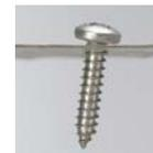
Sheet metal screws with ST threads often lean over as the screw tends to align with the helix angle of the thread - with stripped threads or loose assemblies as a result.
