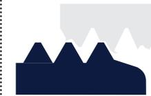
The first thread on a nut is always incomplete, which means there is a risk of cross threading. This risk is generally managed using manual fitting, which is both costly and time consuming.
