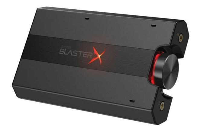
Built with precision audiophile components, the Sound BlasterX G5 is also a 24-bit/192kHz, 120dB USB DAC and headphone amplifier with 2.2 ohm output impedance for high fidelity playback – driving studio-grade headphones up to 600 ohms and sensitive in-ear monitors. The illuminated volume control knob and dedicated SBX and Scout Mode buttons also allow for quick volume or audio adjustments during gaming sessions.
