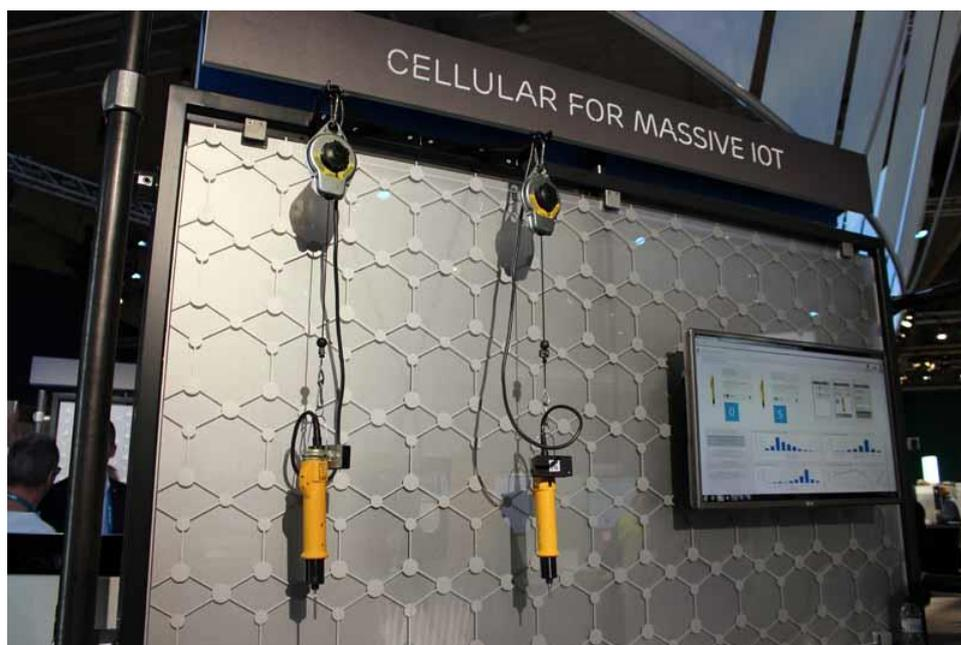
Several low power, wide area (LPWA) use cases are currently being implemented in the factory, such as production line monitoring, warehouse monitoring and package and materials tracking. The centerpiece of the demonstration to be shown in Barcelona is the connected high-precision screwdriver, with motion sensors attached to NB-IoT modules that transmit real-time data of the tools to the Cellular IoT network.
