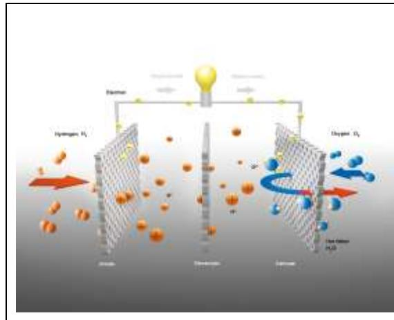
The Viessmann Vitovvalor 300-P converts natural gas into hydrogen; a process that generates both heat and power.
